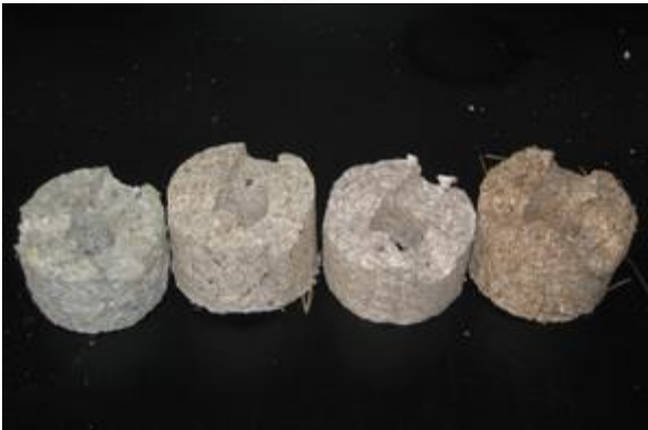
Biomass Packed: Boise State University researchers tested biomass briquettes of four different compositions, left to right, 100 percent paper, 1:3 paper to biomass, 3:1 biomass to paper and 100 percent paper to demonstrate that the energy output of d PHOTO: BOISE STATE UNIVERSITY
