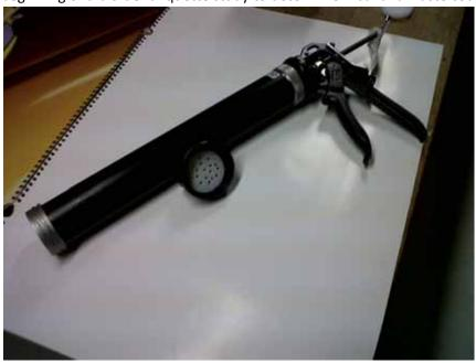
Rwanda where the Greater Cincinnati Professionals Chapter of Engineers without Borders works. The caulk gun used was a COX 51001-2T. It has a solid barrel and is designed for bulk loading. This model has a 26:1 load magnification. This ratio was chosen as it was expected that a normal grip would be around 40 pounds. This would put about 1000 pounds on the area of Pi square inches. The typical 3<sup>rd</sup> world press puts about 2000 pounds on typical
