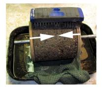
Cover the entire pan with a plastic bag and let cure for approximately 4 days. Open the bag occasionally to check on the progress and to make sure the cloth is wet. After 24 hours you can remove the end caps.
