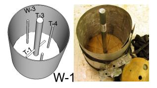
Fill the mold with concrete containing aggregate to about 1 inch from the top.
