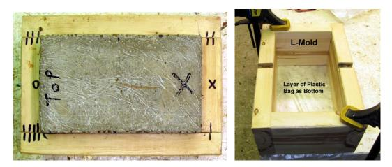
After the no teeth grinding head (NA) has cured for a few days, wrap it tightly in plastic and insert it into the two slots in the L-Mold. Fill the mold with concrete and jiggle to remove air bubbles.
