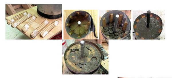
Remove the cylinder when you are comfortable that the concrete has cured sufficiently to be able to wire brush the teeth to expose the aggregate. Do not wire brush the V section of the teeth. Again, keep the end caps in place for about 24 hours until the concrete has cured enough to safely remove them without damaging the edges. Again, cover with a wet cloth and plastic and keep wet for curing.
