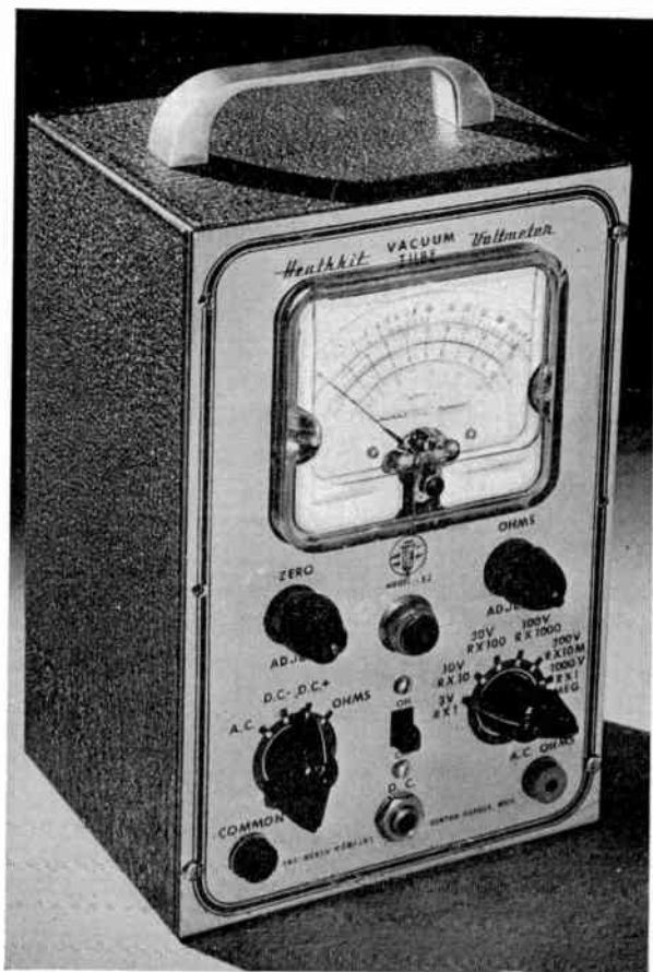
93. Assembly view of Heathkit vacuum-tube voltmeter. ( The Heath Company. )
