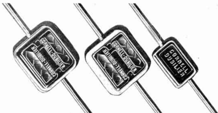
10. Three types of molded-bakelite mica receiving capacitors.
