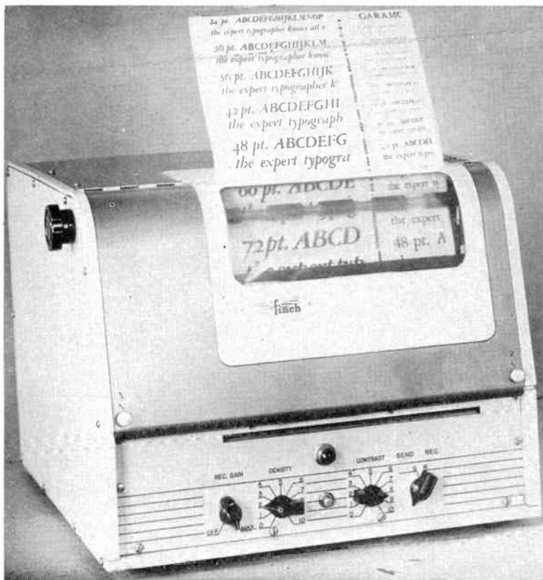
149. The Finch Telefax duplex facsimile unit, a complete sending and receiving machine using radio or wire communication channels. ( Finch Telecommunications, Inc. )
