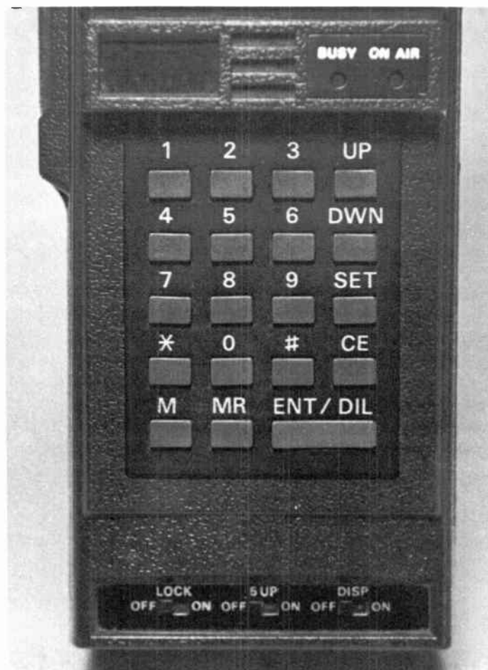
12.1. The 19 push buttons (properly, keys) on the face of the Yaesu Model FT-207R transceiver comprise the nerve center of this typical 2-meter set. Digital readouts of frequency appear in the window at the upper left. After they have been punched in, they can be protected against accidental erasure by the LOCK switch in the lower left corner. CE means correct error ; M, memory ; MR, memory recall ; ENT/DIL enter and display .
