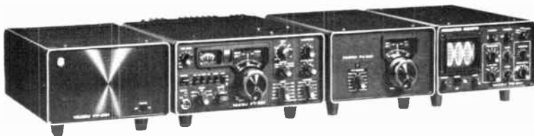
13-7. A stunning lineup of Yaesu equipment of matching design. From the left: FF-301 loudspeaker, FT-301 transceiver, FV-301 variable frequency oscillator, YO-301 monitor scope. Latter permits analysis of transmitted and received signal wave forms.
