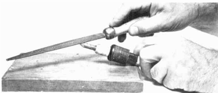
8-13. The tip must be smooth and free of pits. Occasional dressing with a fine file is necessary.
