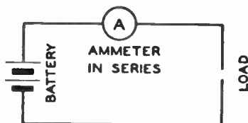
AMMETER CONNECTED IN CIRCUIT
