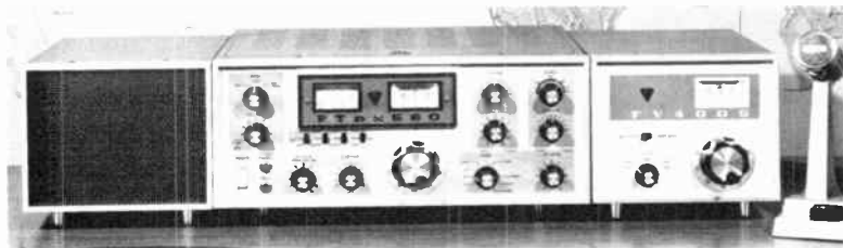
13-8. Another Yaesu array, in a different outward design. From the left: loudspeaker, FTd×560 five-band receiver plus WWV, FV400S outboard variable frequency oscillator for cross-band operation.
