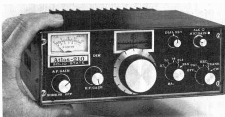
18-2. By contrast, this Atlas-210 all solid-state five-band transceiver is not much larger than a cigar box, and needs little current.
