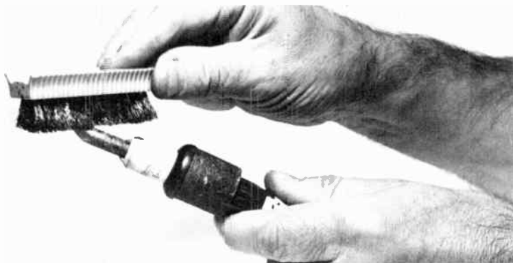
8-12. To keep the tip of the iron free of corrosion, brush it frequently with a brass brush, and apply a dab of solder if necessary to renew
