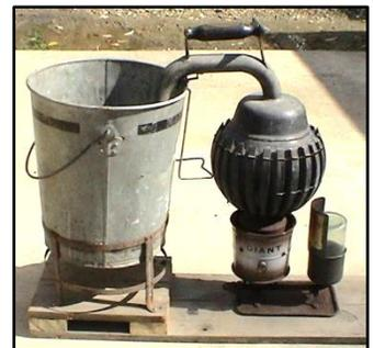
That heat boiled the ammonia to a pressure of 250 psi, pushing the ammonia gas to the smooth ball side, now resting in the bucket of water where it condensed into a liquid. Water remained in the hot ball because ammonia has a lower boiling point than water.
