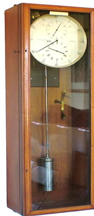
Clocks manufactured by James Ritchie & Son, Edinburgh, Scotland, were acquired with one clock for the Carlisle Building and a second clock as an upgrade to the observatory's master clock in 1873. Photo by L. Hite
