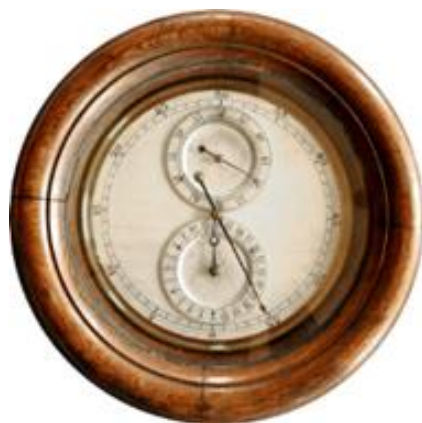
The Hipp Observatory (slave dial) clock from Peyer Favarger & Co. was controlled by the Riefler slave clock in the master clock vault and was visible to the astronomer operating the Meridian Circle Telescope.
