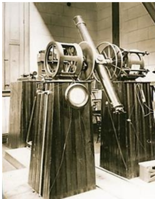
The Fauth & Co. Meridian Circle Telescope, located in the transit viewing room, is mounted to cast iron piers and features the Hipp Observatory (slave dial) clock attached to the front left-hand pier. Image from COC
