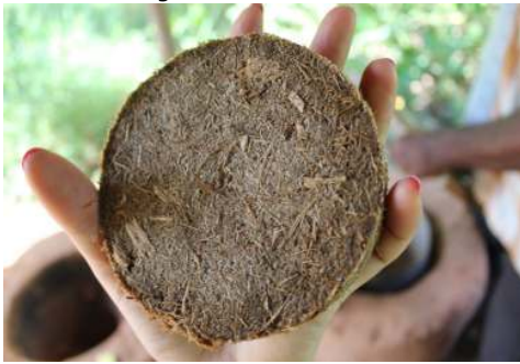
Figure 1: Image of bagasse pith briquette made on car-jack press constructed in Puducherry
