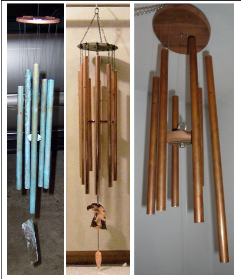
Figure 2: Three examples of student wind chimes. All three of these chimes are made using copper tubing. The picture on the right shows a typical basic set of chimes. In the middle picture there are two chimes for each note and some very detailed work on the sail. The left hand set of chimes had a chemically accelerated patina.
